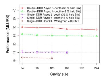
Figure 9. OPAL\_async vs. OPAL OpenCL on MPPA for duration = 1000 steps.
