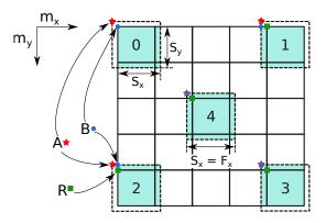
Figure 8. Local/Remote copied index in 2D (in lattice node) with A: begin of the local buffer = (0,0); R: begin of the remote main block cuboid (without halo); B: begin of the copied cuboid (S), represented by:  $B_a$ : index of S on local memory (from A) and  $B_r$ : index of S on global memory (from R).
