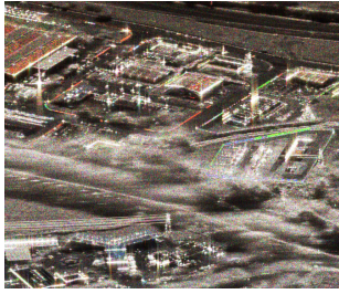
Fig. 2. An ONERA RGB color-coded SAR image acquired for three consecutive spectral sub-bands.
