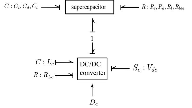
Fig. 5. Bond Graph Model of the supercapacitor system.
