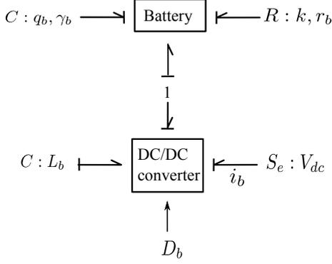
Fig. 4. Bond Graph Model for the battery system
