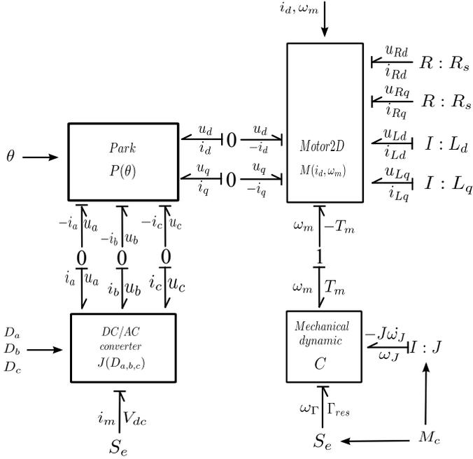
Fig. 3. Bond Graph Model for the electromechanical sub-system
