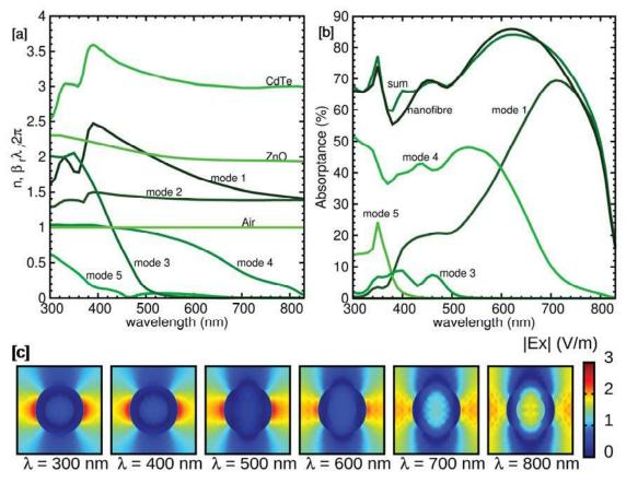
Fig. 4. (a) The real part of the normalized propagation constant (i.e.  $\beta_r \lambda / 2\pi$ ) and (b) the absorptance for the 5 selected optical modes found for the optimal geometrical dimensions with D = 200 nm and P = 350 nm. The real part of the refractive indices (i.e. *n*) for ZnO and CdTe is also reported in (a) for comparison. (c) Maps of the modulus of the electric field  $E_x$  for the optical mode 4 for various wavelength
