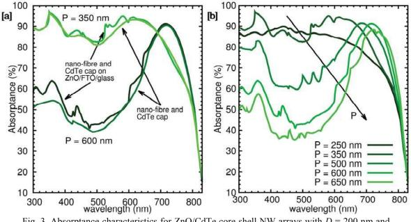
Fig. 3. Absorptance characteristics for ZnO/CdTe core shell NW arrays with D = 200 nm and various periods (i.e., set of geometrical dimensions A).
