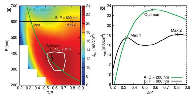
Fig. 2. (a) Ideal  $J_{sc}$  map as a function of *P* and *D*/*P*. (b) Ideal  $J_{sc}$  as a function of *D*/*P* for the two sets of geometrical dimensions A and B.
