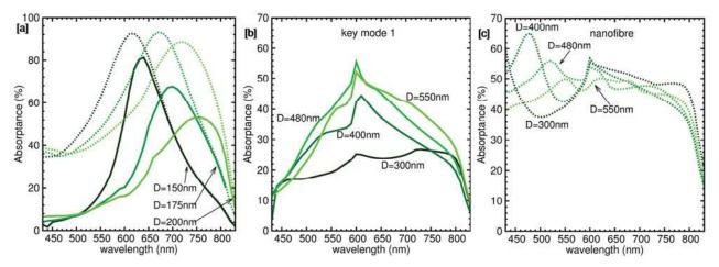
Fig. 7. Absorptance of the key optically guided mode 1 (solid line) and of the ZnO/CdTe nanofibre arrays (dotted line) for the set of geometrical dimensions B (i.e., P = 600 nm and different values of D). (a) For D = 150, 175, 200 nm and (b-c) for D = 300, 400, 480, 550 nm.
