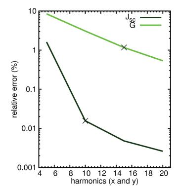
Fig. 9. Convergence of both the ideal  $J_{sc}$  and the surface integrated generation rate G versus the harmonic number for both Fourier series. It has been calculated for the ZnO/CdTe NW arrays with P = 350 nm and D = 210 nm. The reference value is calculated with 25x25 harmonics.
