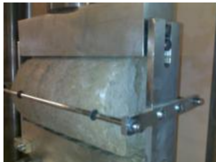
Figure 5 Brazilian test to determine the tensile strength
