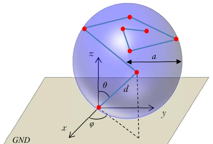
**Figure 1.** Shematic representation of a crooked wire antenna having 7 wires.
